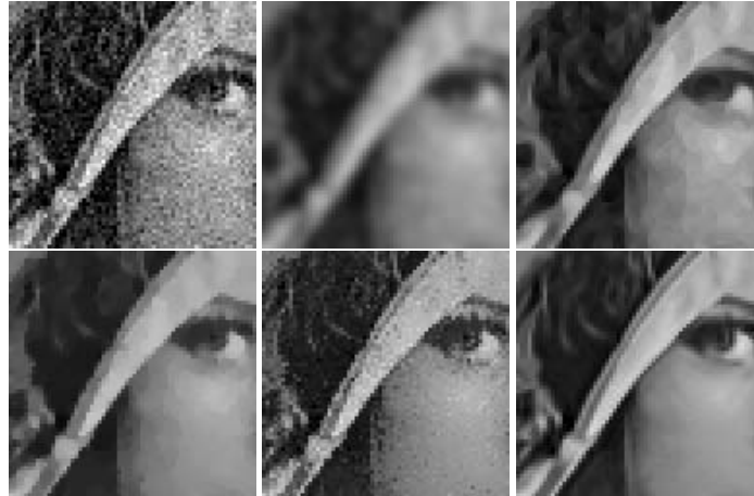
Figure 5. Denoising experience on a natural image. From left to right and from top to bottom: noisy image (standard deviation 20), Gauss filtering, anisotropic filtering, Total variation, Neighborhood filtering and NL-means algorithm. The removed details must be compared with the method noise experience, Figure 4.
